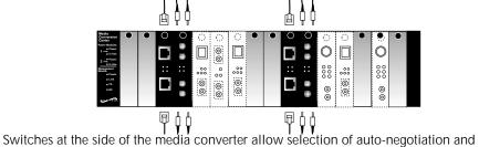
Switches at the side of the media converter allow selection of auto-negotiation and of full/half-duplex. Also, a port select timer (PST) switch\* allows the network administrator to set different timer values (used when a primary connection is lost and a secondary connection is made) at each end of the copper/fiber interface.
